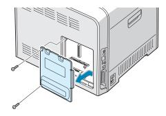
4 Locate the memory DIMM slot (the upper slot) on the control board.
